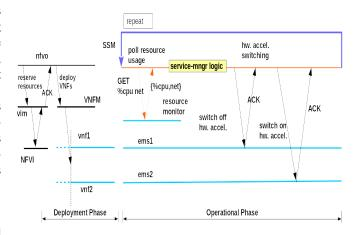
Fig. 2. Components and NFV processes involved in the accelerator allocation scheme.
