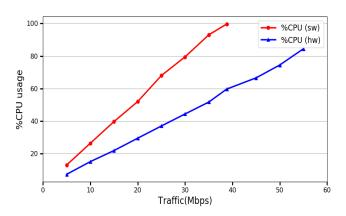
Fig. 5. Variation of %CPU usage of SSH-clients VNFS with changing traffic for non-accelerated (sw) and accelerated modes (hw).
