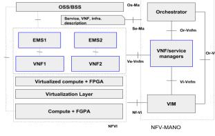
Fig. 1. ETSI's reference architecture for NFV.
