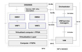
Fig. 1 ETSI NFV reference architecture framework.
