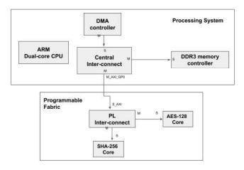
Fig. 3 System design for hardware acceleration of AES128 and SHA256.
